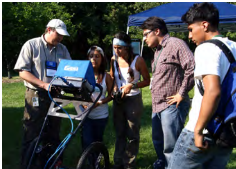
Edwin Muñiz, NJ Assistant State Soil Scientist, explains how ground penetrating radar is used in soil survey while students receive hands-on experience.
